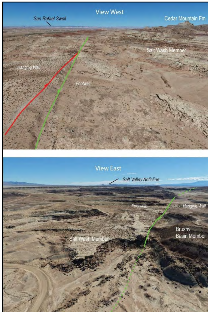
Figure S5C-3. Drone views east and west along the northern bounding fault of the Ten Mile Graben taken from the road. Drone photograph by R. Cole. Mode I fractures are clearly visible across the Salt Wash sandstone.
